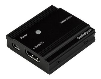
This 4K HDMI signal booster lets you increase the signal strength of your HDMI video source so it can travel greater distances using standard HDMI cables. You can achieve resolutions up to 4K at 60Hz at distances of up to 30 ft. (10 m), and depending on your desired resolution, the booster supports distances up to 115 ft. (35 m) away at 1080p 60Hz resolution.
